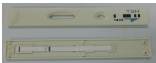
Figure 1. The representative appearance of FL immunochip for TSH. Scanning window (left oval circle), sample loading well (right round circle) and insertion arrow into scanner are seen from the top panel of the immunochip. The nitrocellulose membrane strip immobilized with anti-TSH-mAb and chicken IgY is lied on the bottom panel. Sizes of strip and immunochip, and amounts of Abs immobilized were described in details at the section of strip, immunochip, and scanner in Materials and Methods.
