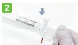
Place the C-tip in the cartridge tip hole and insert the cartridge into the slot
